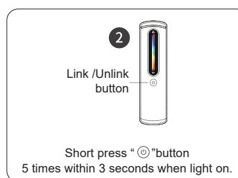
Short press "Link /Unlink" button 5 times within 3 seconds when light on.
