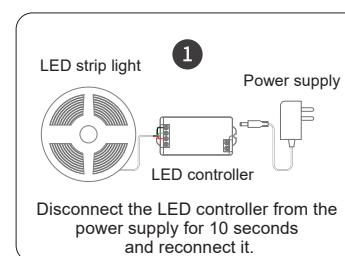
Disconnect the LED controller from the power supply for 10 seconds and reconnect it.
