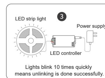
Lights blink 10 times quickly means unlinking is done successfully.
