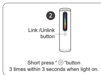
Short press "Link /Unlink" button 3 times within 3 seconds when light on.
