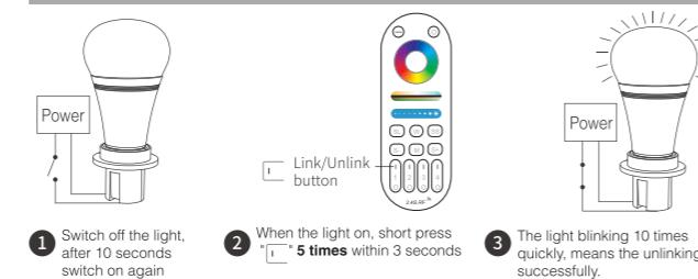
If the light not blink quickly, the unlink failed, pls switch off the light again, and follow the above steps to unlink again.
