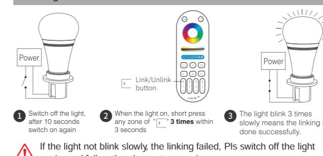
If the light not blink slowly, the linking failed. Pls switch off the light again, and follow the above steps again.
